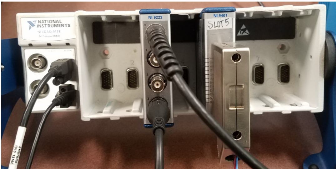
Figure 3: National Instruments Data Acquisition Setup
